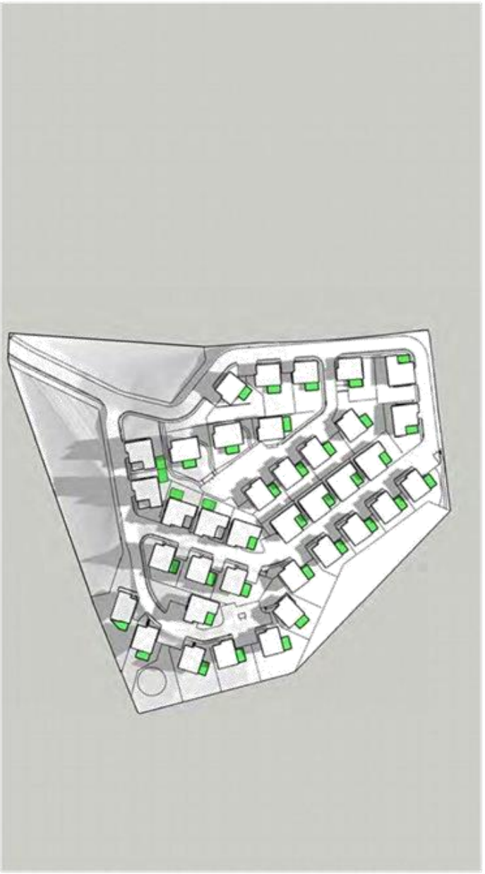
SITE SHADING - PLAN VIEW - 12pm JUNE 21 SCALE: NTS
