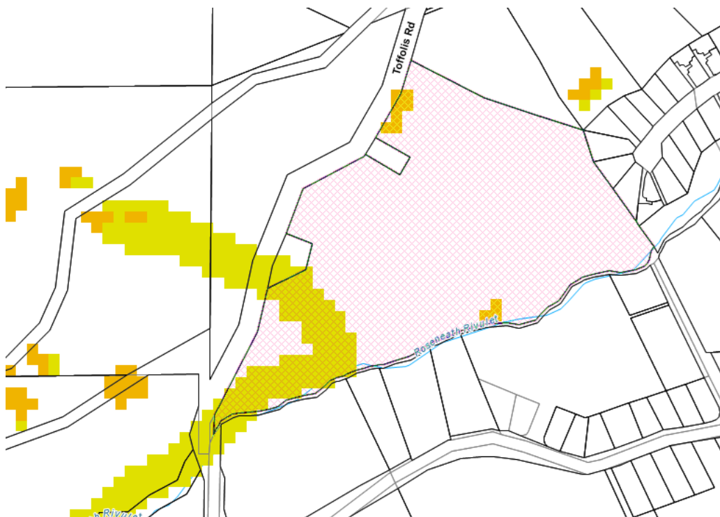
Figure 8: An extract of exponare to show the extent of the Landslide Code (Yellow – Low Landslide Hazard Area; Orange – Medium Landslide Hazard Area)
