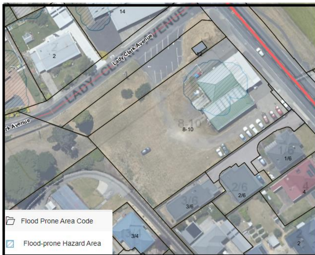
Figure 8 – Extent of flood-prone hazard area overlay
