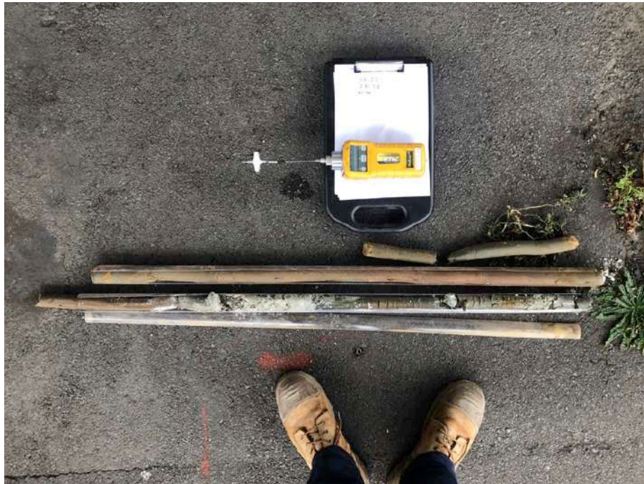
Push tube sample from MW01 1.8-3.8 mBGS showing shallow sandy CLAYS moving into clayey SAND with gravel. Note that the top of core at the top left of image and the bottom at the bottom right.
