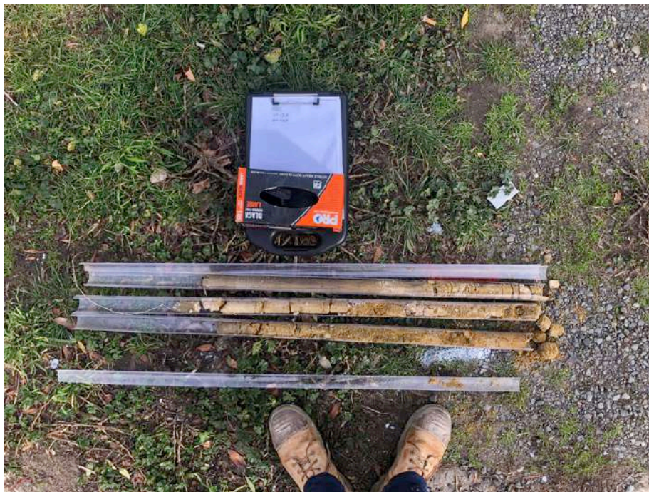
Push tube sample from MW02 1.1-3.6 mBGS. Note the SAND dominant material is shallower than in MW01 and that the top of core is at the top left of the image and the bottom at the bottom right.
