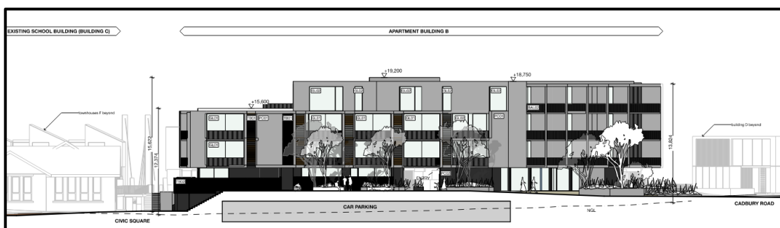
Figure 4. A view of the northern elevation of Building B showing the reduction in scale in proximity to the existing school building.
