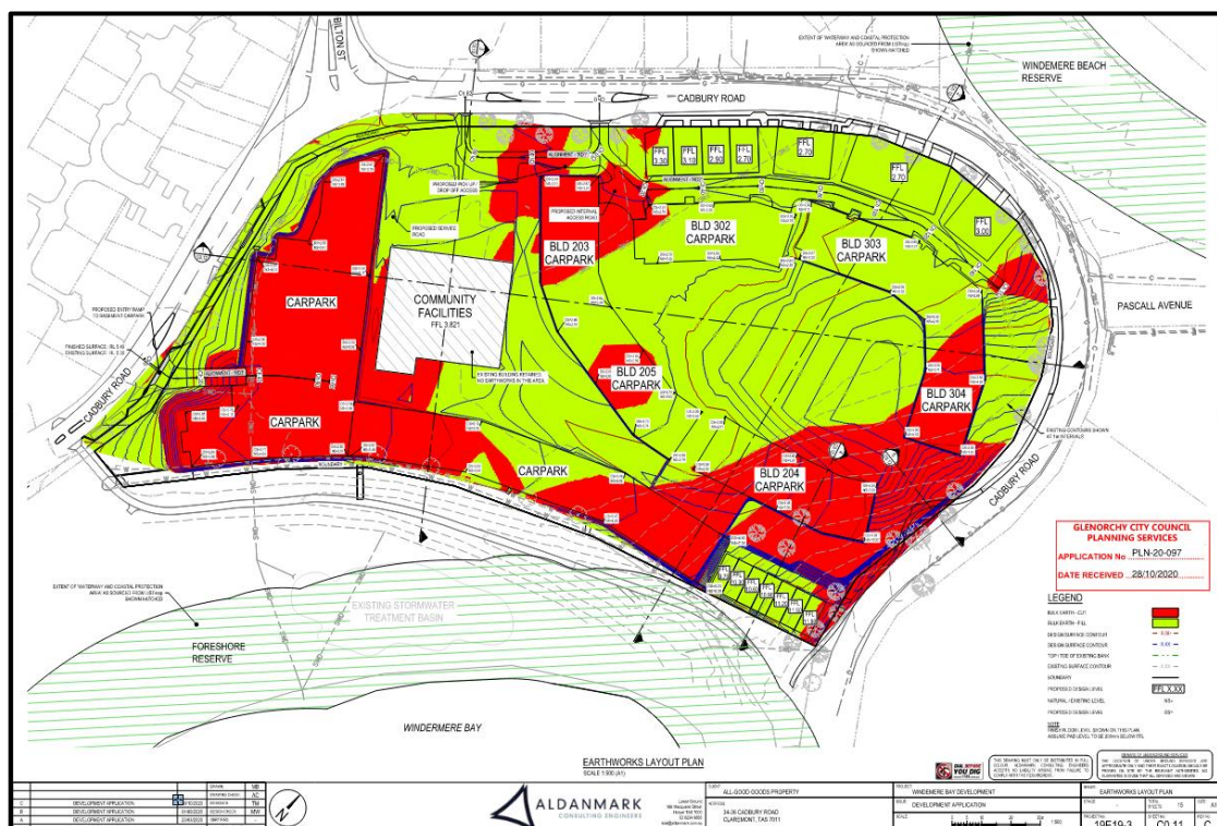
Figure 19. The layout plan for earthworks on the site to facilitate the development.
