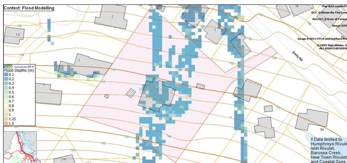
Figure 5 – The site is identified as being subject to flood risk (blue/green – Council database 2020 (Exponare Flood Modelling Context))
