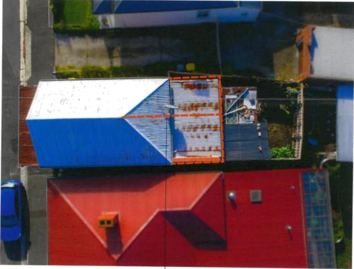
Continue ridge line of existing roof.
