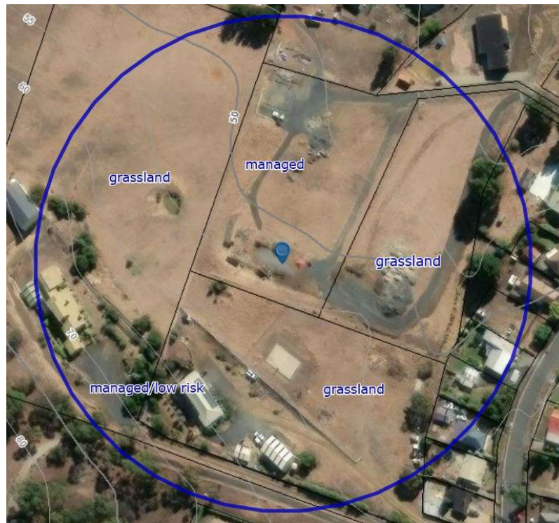
Aerial view showing 120m radius from proposed dwelling. Neighbouring properties consisting of managed lawns and gardens around the dwellings with surrounding paddocks assessed as grassland.
